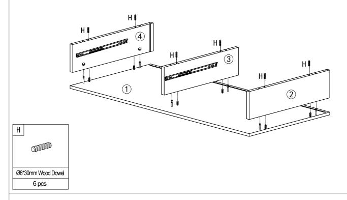
3. Attaching the Bottom Panel to the dressing table frame.
