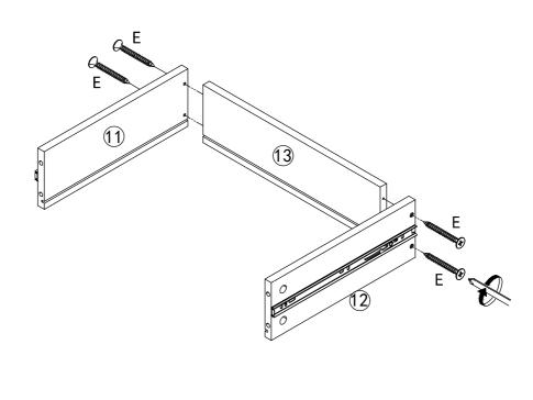
8. Attaching the Drawer Bottom Panel to the Drawer frame.
