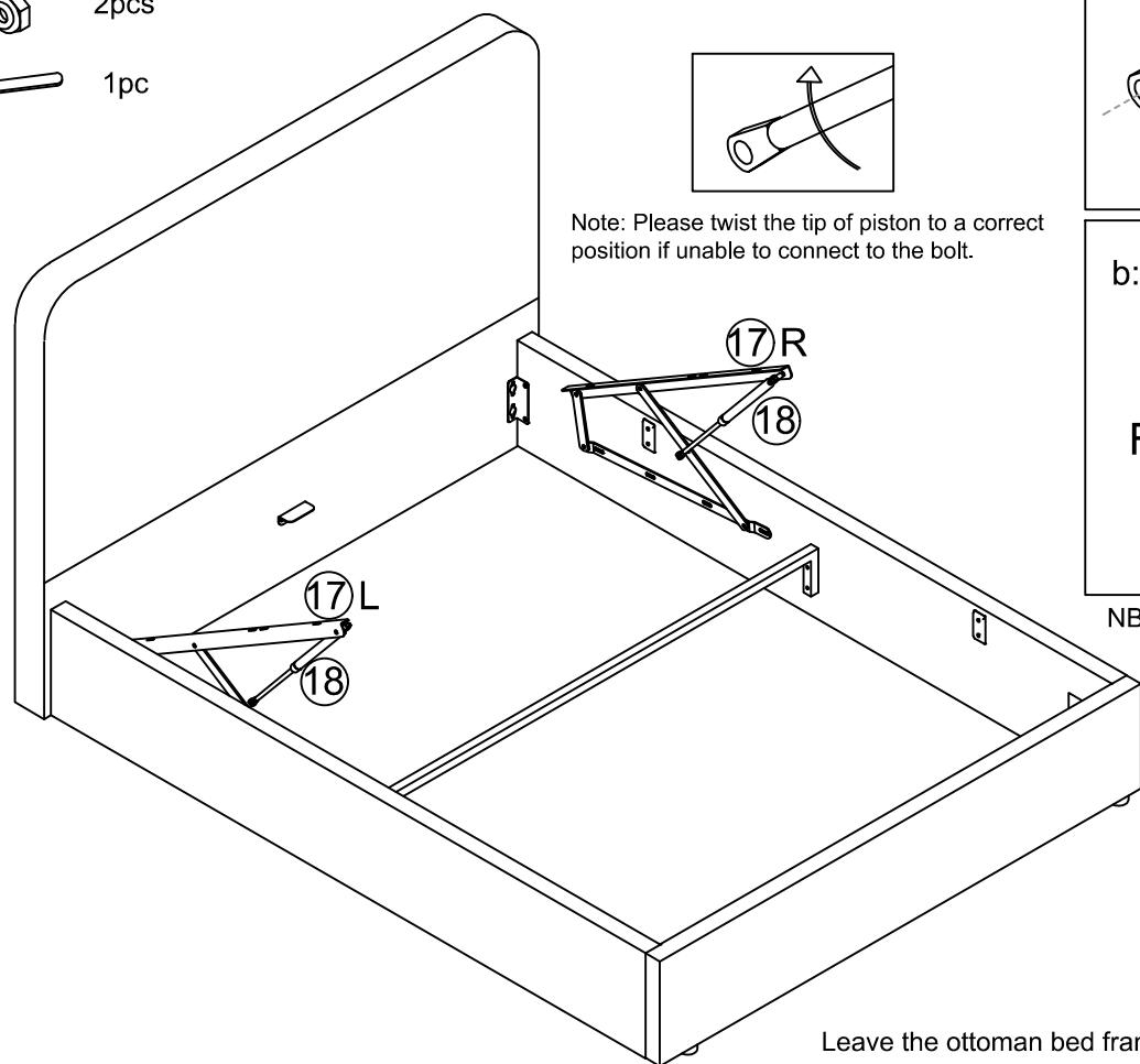
Note: Please twist the tip of piston to a correct position if unable to connect to the bolt.
