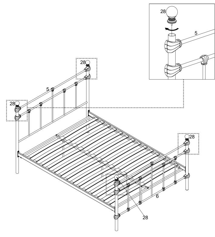
▲ Interior legs intentionally do not touch the ground. This will provide additional support and help protect your bed from damage.
