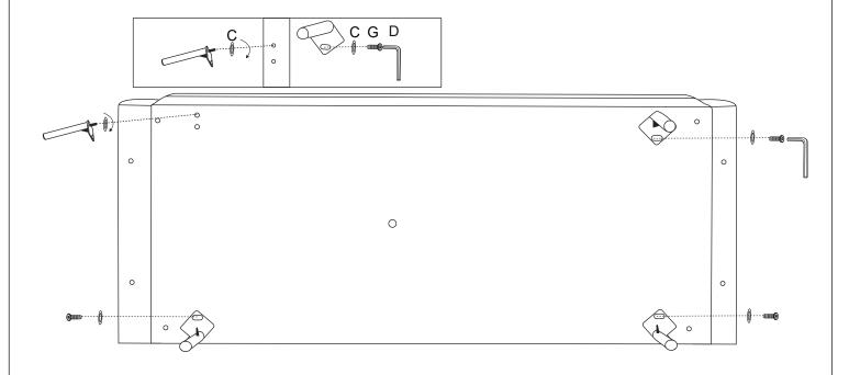
Step 4: Attach the legs (A, K& E) to the underside of the sofa using 8x screws (F) and 8x washer(C) on each side, being sure that leg (A) are at the front and (K) is at the back.
