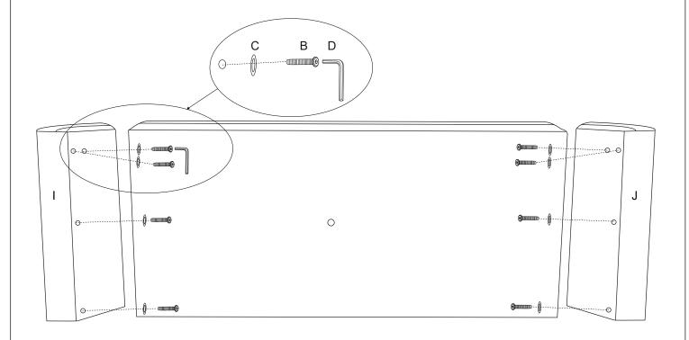
Step 3: Use the 4 screws (G) and 4x washer(C) on each side to attach the base frame (A) to the bottom of the sofa.
