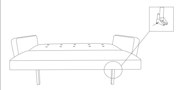
Step 7: To convert from the sofa bed to the sofa position, collapse the legs by pressing the latch at the top of the legs on the left hand side, being careful not to trap your fingers, fold the legs in and zip up the zipper. lift the sofa backrest and push it toward the front of the sofa until both sides click.
