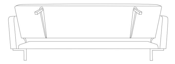
Step 6: To convert from the sofa position to the bed position, pull the backrest towards the front of the sofa until both the left and right side have clicked. proceed to lower the backrest down into the horizontal position.
