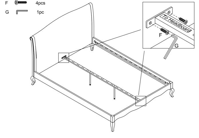
Step 5: Attaching the Slat Caps & Slats to the Bed Frame
