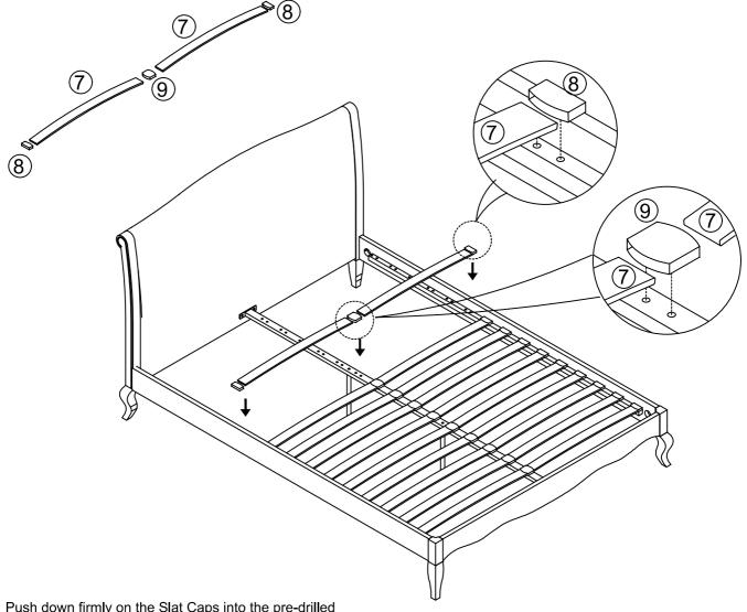
Push down firmly on the Slat Caps into the pre-drilled holes on the Side Support Rail & Central Support Rail. It is recommended to push the Centre Slat Caps into position before pushing down on the Side Slat Caps.
