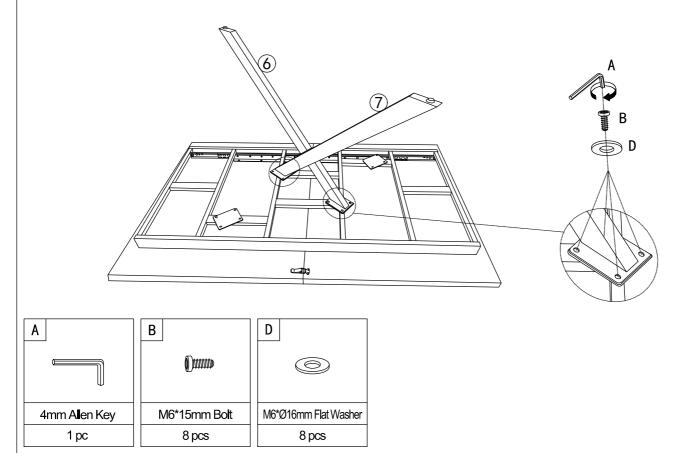
7. Attaching the Long Leg A and the Long Leg B to the Iron Frame, and apply the foot pads on.
