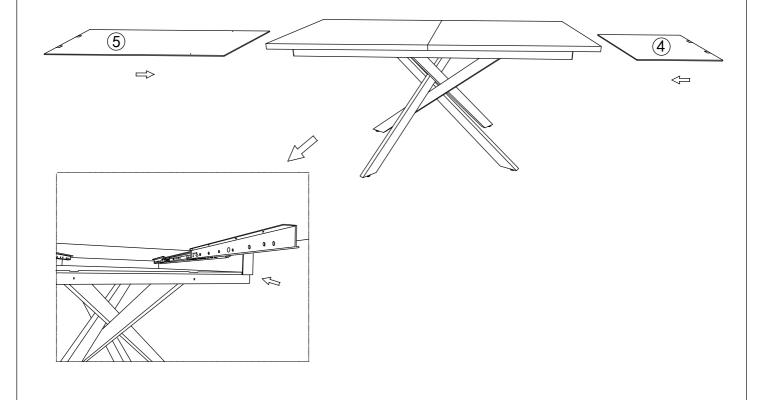
9. Attaching the Bracket to secure the two Carry panels.
