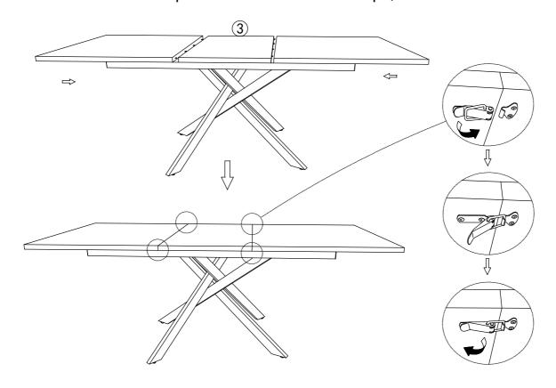
13. Put the Middle Top inside the iron frame, and place to the storge room under the top.
