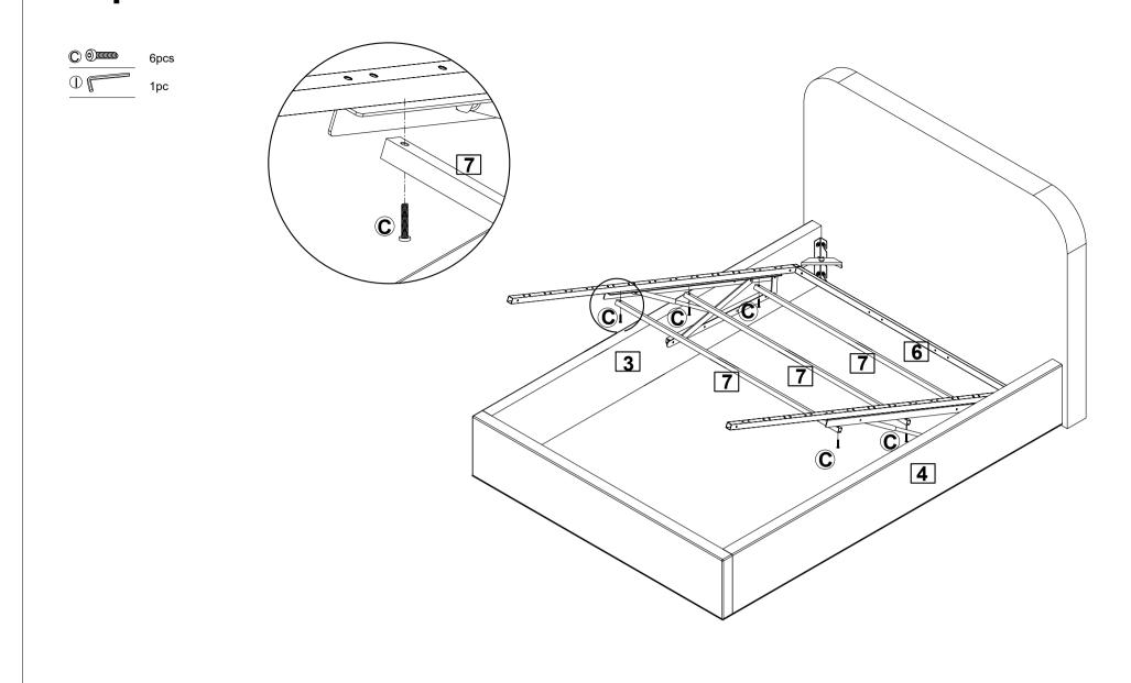
Step 9: Attaching the Centre Support Rails to the Rear Ottoman Metal Frame
