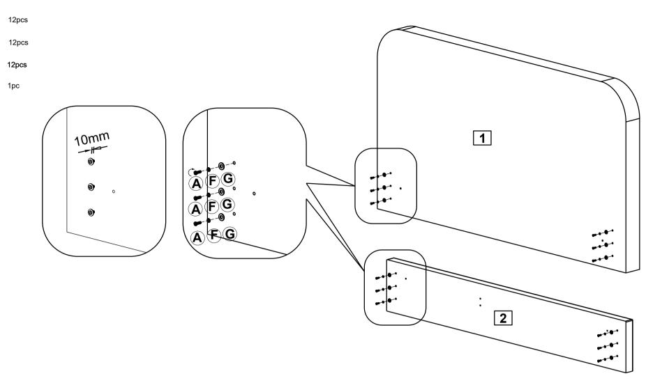
Step 3: Attaching the Left & Right Side Rails to the Headboard & Footboard
