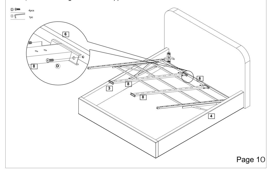
Step 10: Attaching the Central Support Rails & Side Rails to the Front Ottoman Metal Frame
