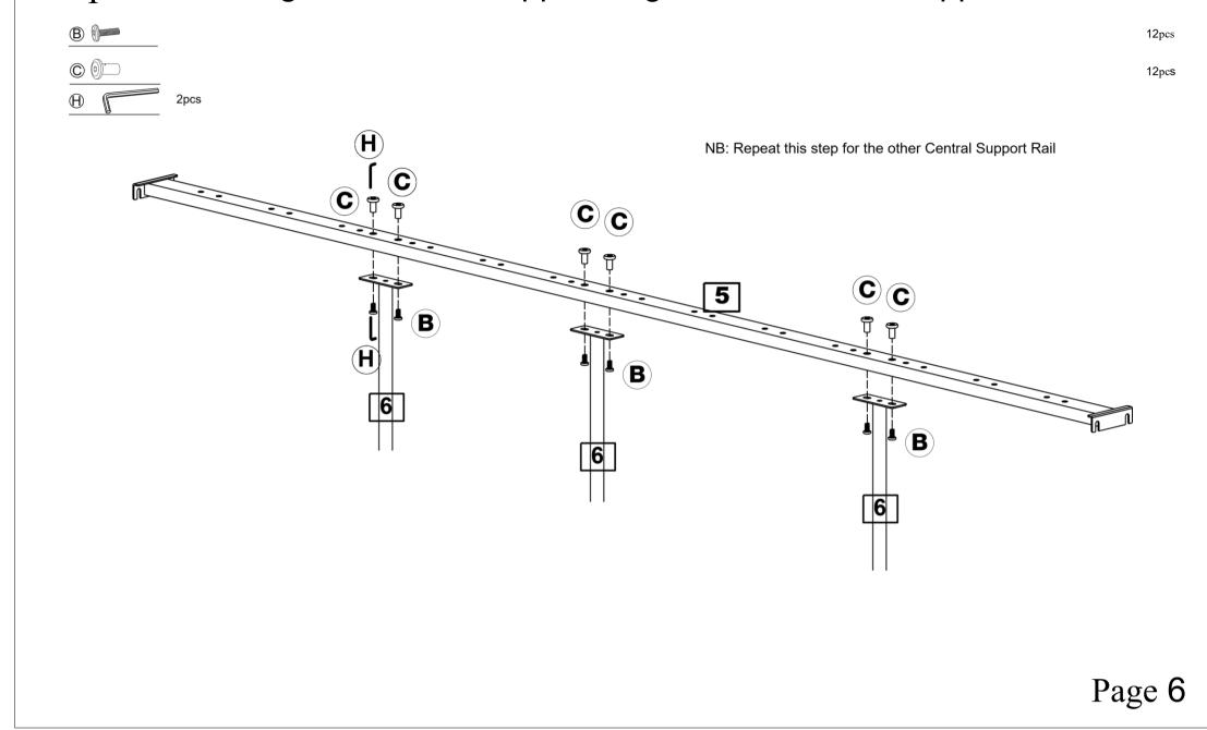
Step 5: Attaching the Central Support Rail to the Headboard & Footboard
