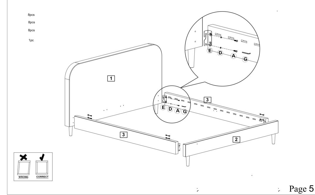
Step 3: Attaching the Horizontal Support Rail to the Side Rails 4pcs 1рс 1
