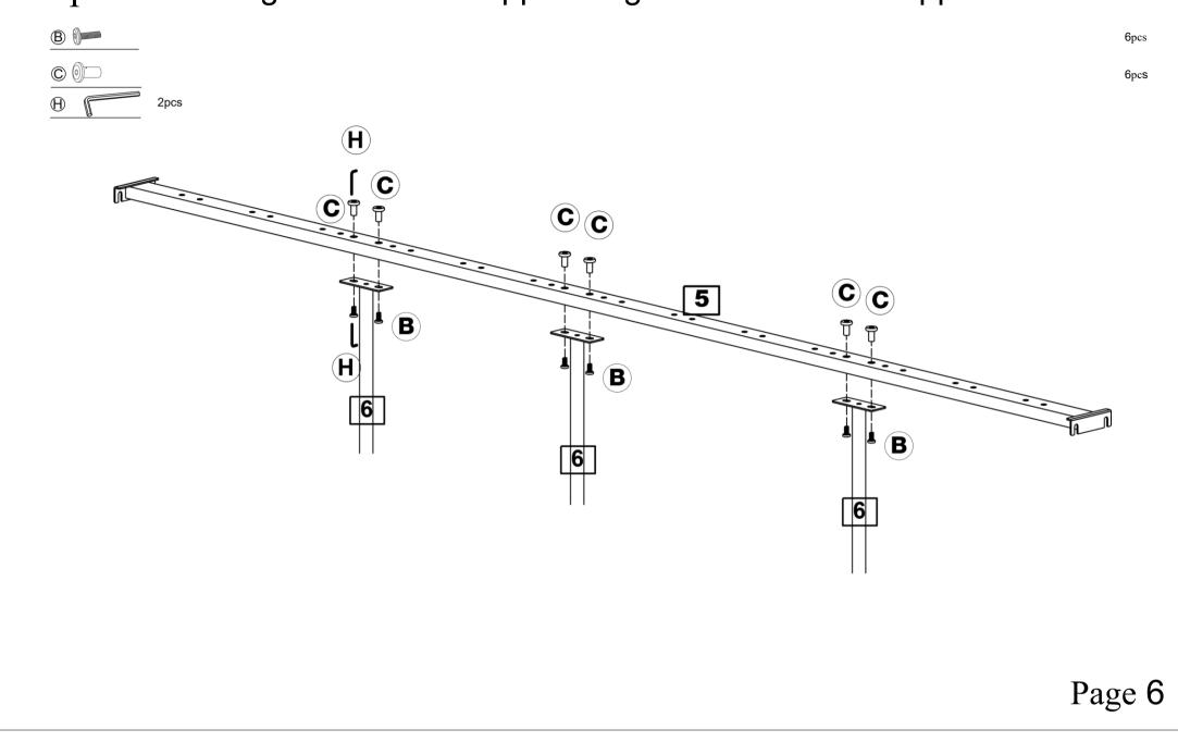
Step 5: Attaching the Central Support Rail to the Headboard & Footboard
