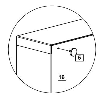
Attach the Legs (5) to the base and tighten.
