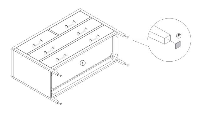
**Step 2:** Disassemble the pre-attached handles and re-attach as shown in the figures.
