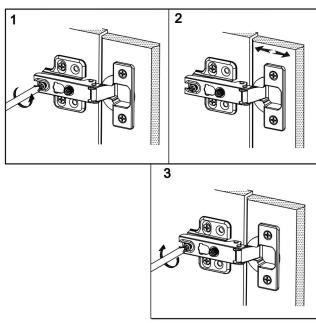
Once flaps have been adjusted vertically. Fit screws (E) to fix plates (K) in their final position.
