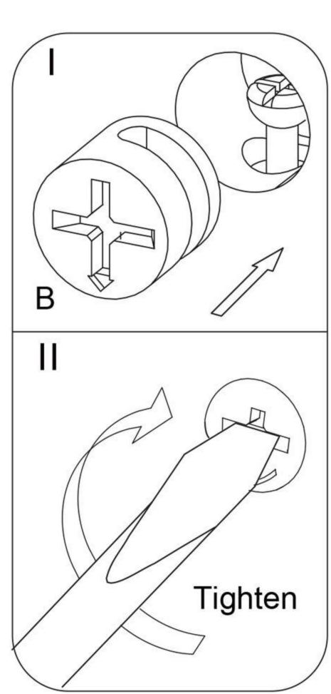
**Step 5** 1.Attach End Cross Bar to the Bottom Panel. 2.Attach CAM Bolts.
