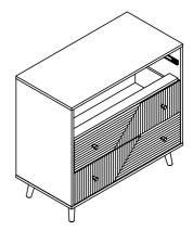
Manually adjust the frame slightly to ensure the drawers are in the correct position, even and parallel before attaching the plastic buckles.
