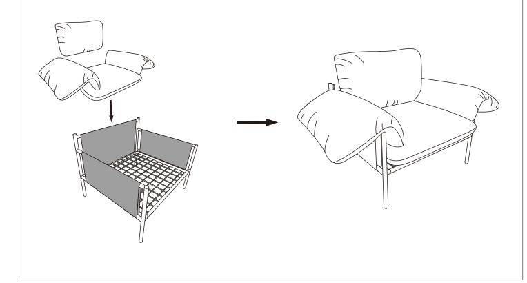
Step 5: Put the assembled chair onto a flat base and then fully tighten all bolts 100%
