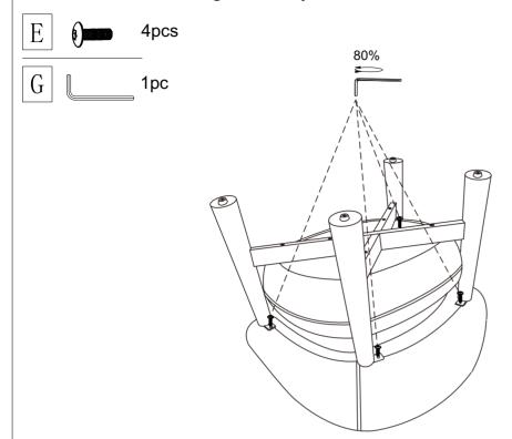
Step 3: Put the assembled chair onto a flat base and then fully tighten all bolts. 100%
