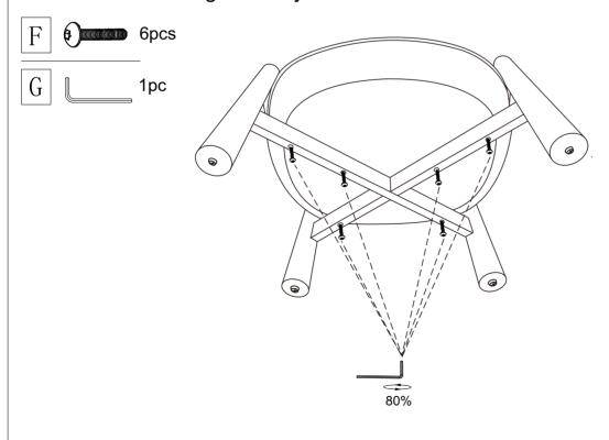
Step 2:Assemble Leg C and D to Backrest B . Remember do not tighten fully until the structure is assembled.
