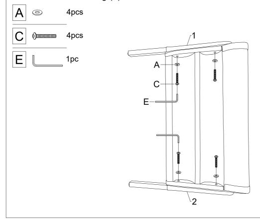
Step 3: Then back to the seat, screw the other side leg (1) to the seat, then close the velcro. 9 3pcs В 3pcs 1рс В E Step 4: Attach the metal bar (3). e 2pcs Ε 1pc
