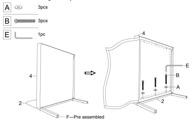
Step 2: Pull the velcro strap on the back, screw one side of the back first, meanwhile, attach the other side leg (1) to the seat. screw the other side back, then close the velcro.
