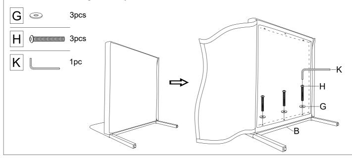
Step 2: Pull the velcro strap on the back, screw one side of the back first, meanwhile, attach the other side leg (A) to the seat. screw the other side back, then close the velcro.
