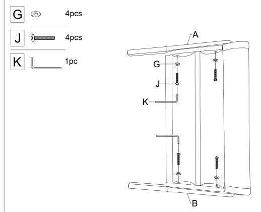
Step 3: Then back to the seat, screw the other side leg (A) to the Seat.
